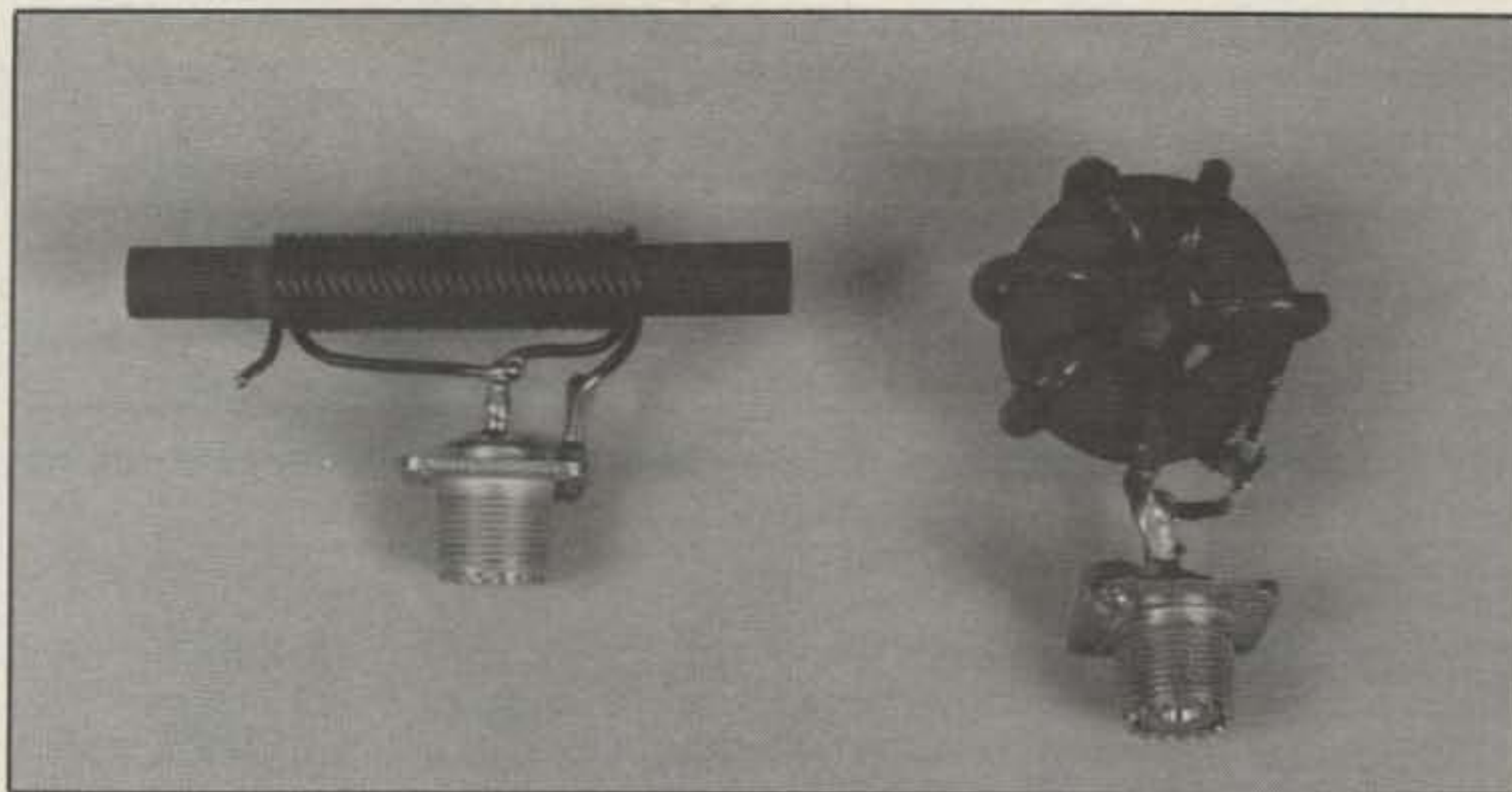
Photo A— Two versions of the Ruthroff 4:1 (50:12.5 ohm) unun: coiled wire rod (on the left); coiled coaxial cable toroid (on the right).
